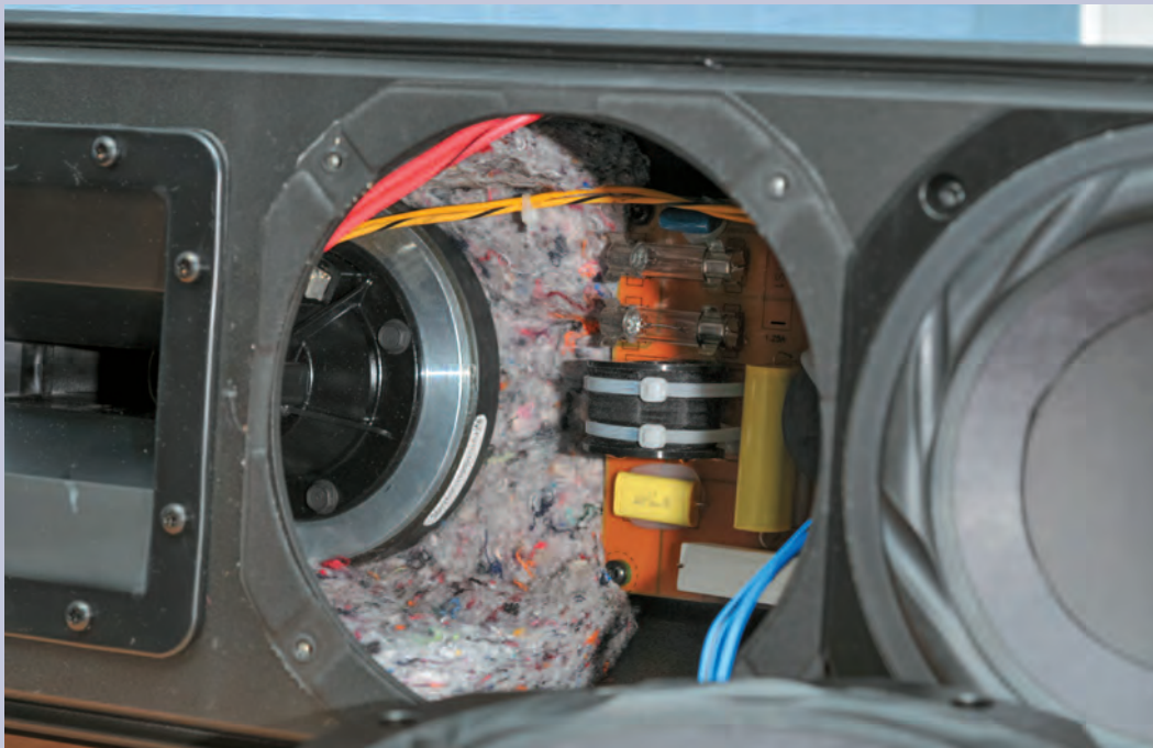
The slightly recessed EV DH-3 1" HF driver
