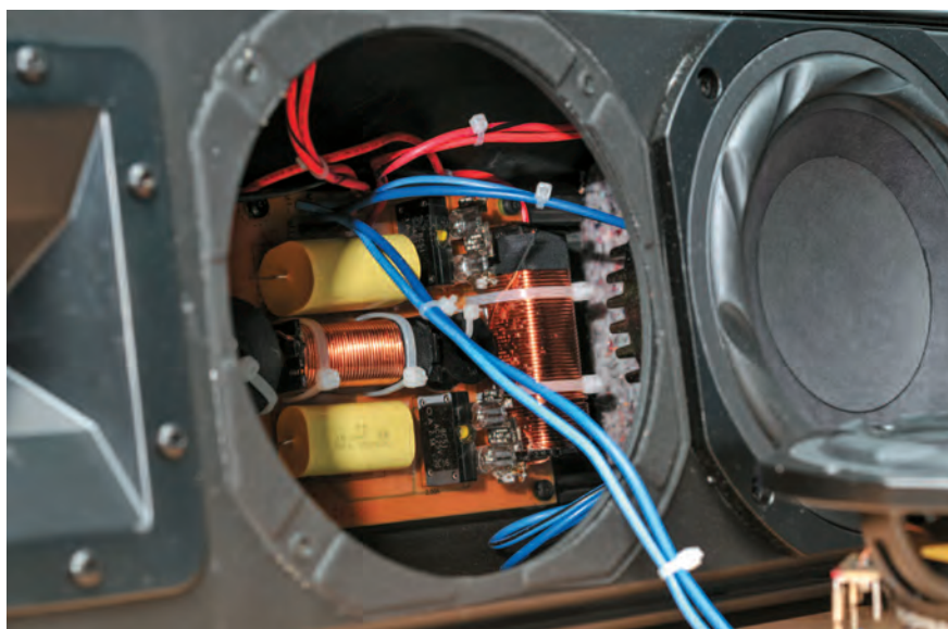
Looking into the interior of the TS400 at the generously dimensioned passive crossover with light bulbs for overload protection. The housing is constructed from an aluminium strand-cast profile
