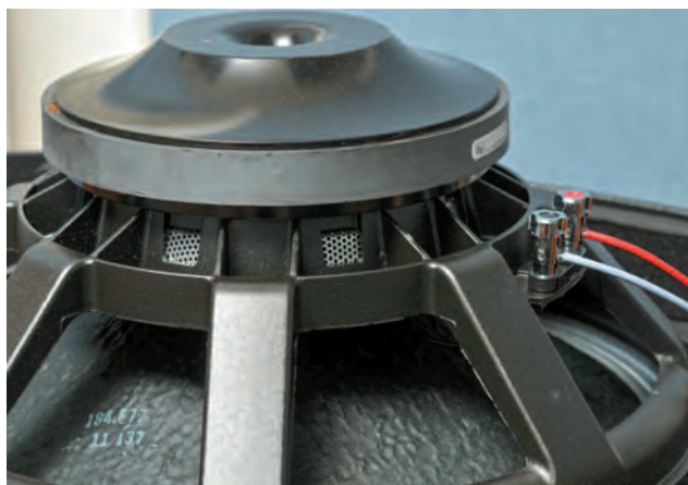
15" driver from EV in the PSD15. Clearly recognizable are the voice-coil vents with their tiny grilles to prevent dirt getting in
