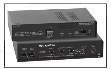
**APPLICATION:** The SF-MA100A is an audio power amplifier that receives three audio channels on an RJ45 Format-A connector. The three inputs are mixed either by the three rear-panel potentiometers or remotely by the three potentiometers on the remote control (available separately). Local or remote control is defined by the Mode switch on the rear panel. If the mixer is remote-controlled, the rear-panel potentiometers set the maximum gain applied to each input.
